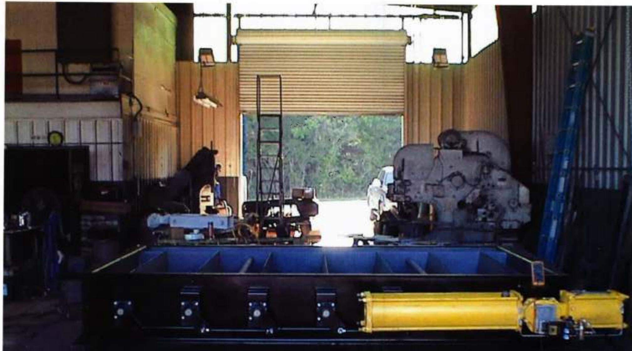
Boiler outlet dual compartment parallel blade louver damper designed for modulating service to proportionally control or isolate outlet gas flow. Damper complete with spring-return pneumatic scotch yoke actuator, electro-pneumatic positioner and remote end-of-travel switch.
