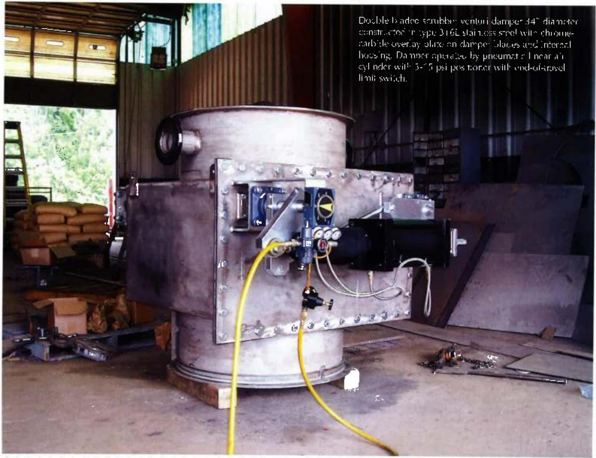
Double blade scrubber venturi damper 34" diameter constructed in type 316L stainless steel with chrome-carbide overlay plating on damper blades and internal housing. Damper operated by pneumatic linear air cylinder with 3-15 psi positioner with end-of-travel limit switch.
