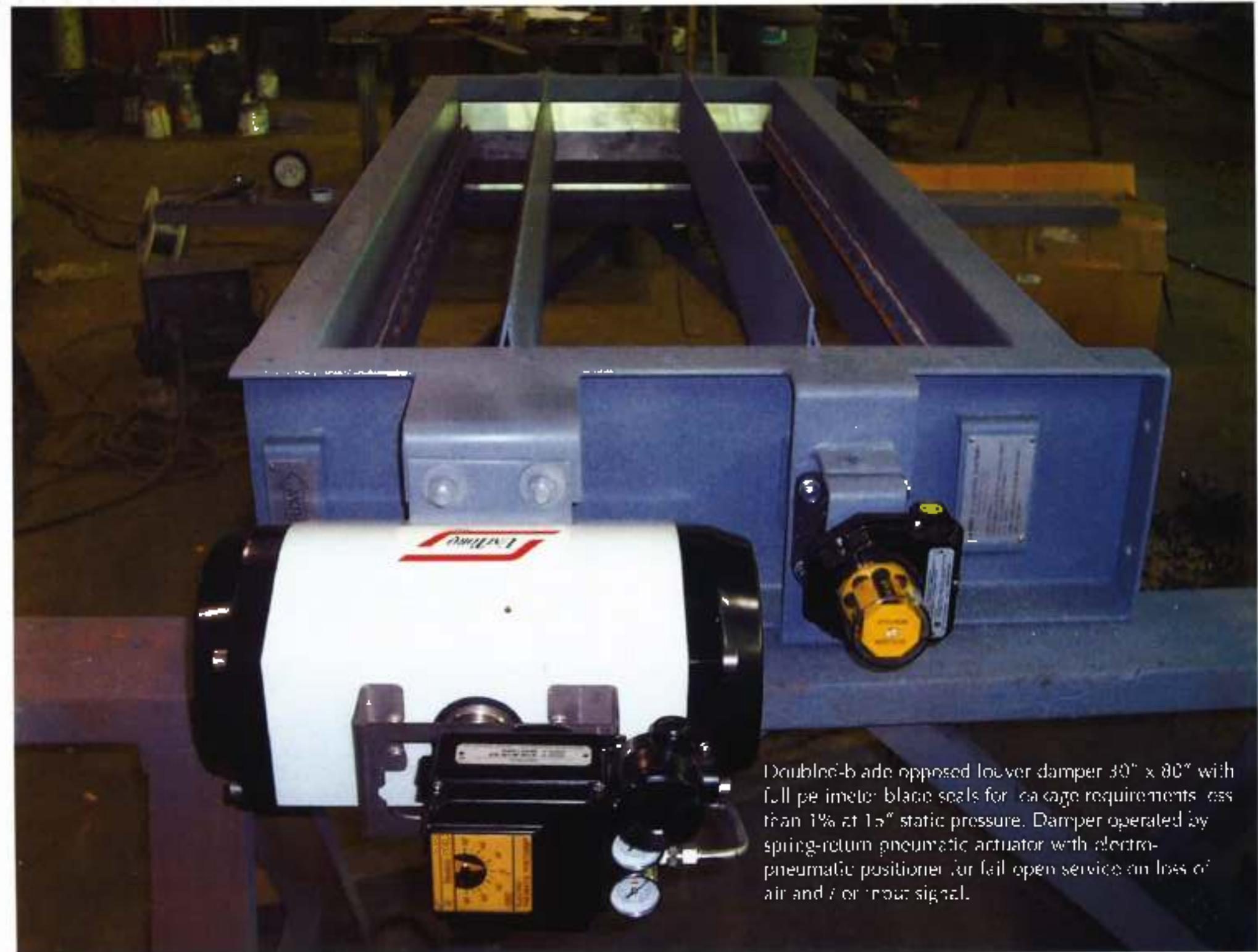
Double-blade opposed louver damper 30" x 80" with full perimeter blade seals for leakage requirements less than 1% at 1.5" static pressure. Damper operated by spring-return pneumatic actuator with electro-pneumatic positioner for fail open service on loss of air and / or trout signal.
