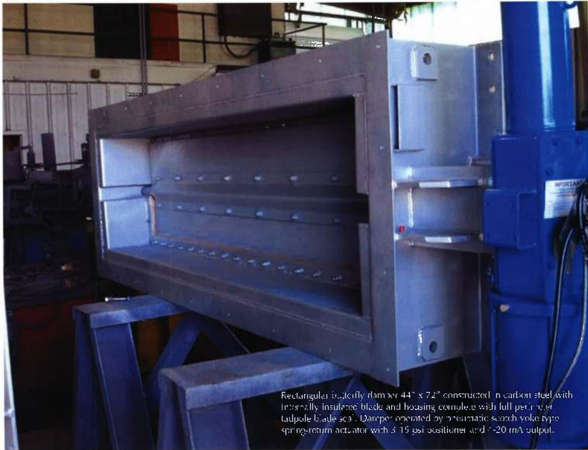
Rectangular butterfly damper 44" x 72" constructed in carbon steel with internally insulated blade and housing complete with full perimeter tadpole blade seal. Damper operated by pneumatic scotch yoke type spring-return actuator with 3-15 psi positioner and 4-20 mA output.
