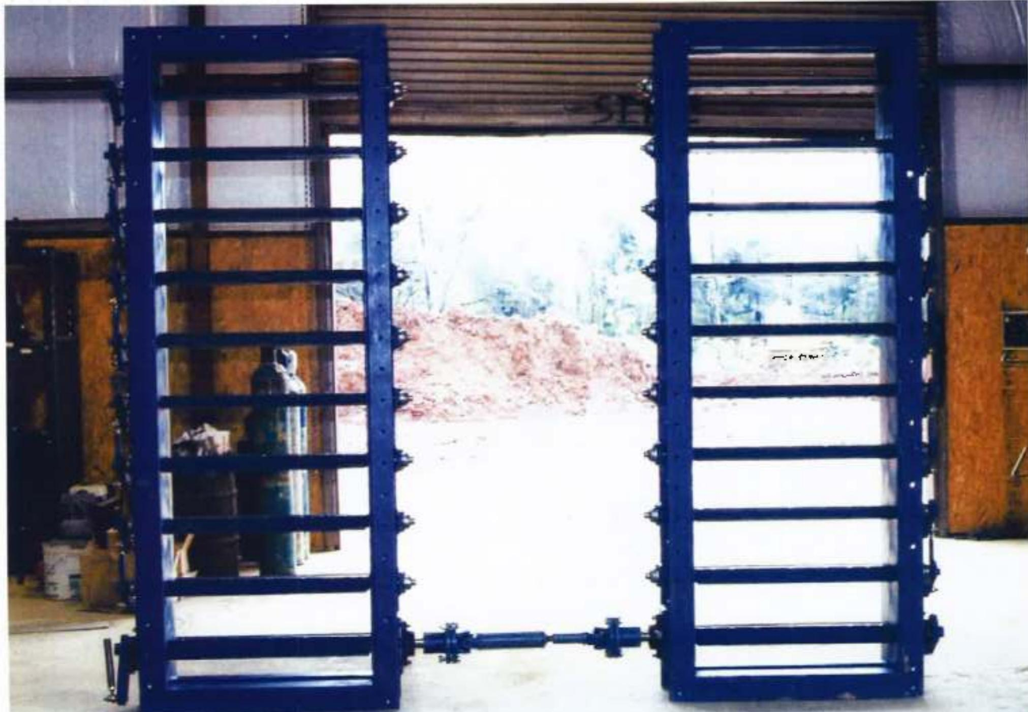
Multi-louver parallel blade inlet dampers 34" x 102" for double width lime kiln ID fan complete with adjustable crossover drive shaft. Damper frame lined with abrasion resistant plate. Damper airfoil blades constructed in abrasion resistant plate. Damper designed for fan start-up at 88" static pressure.
