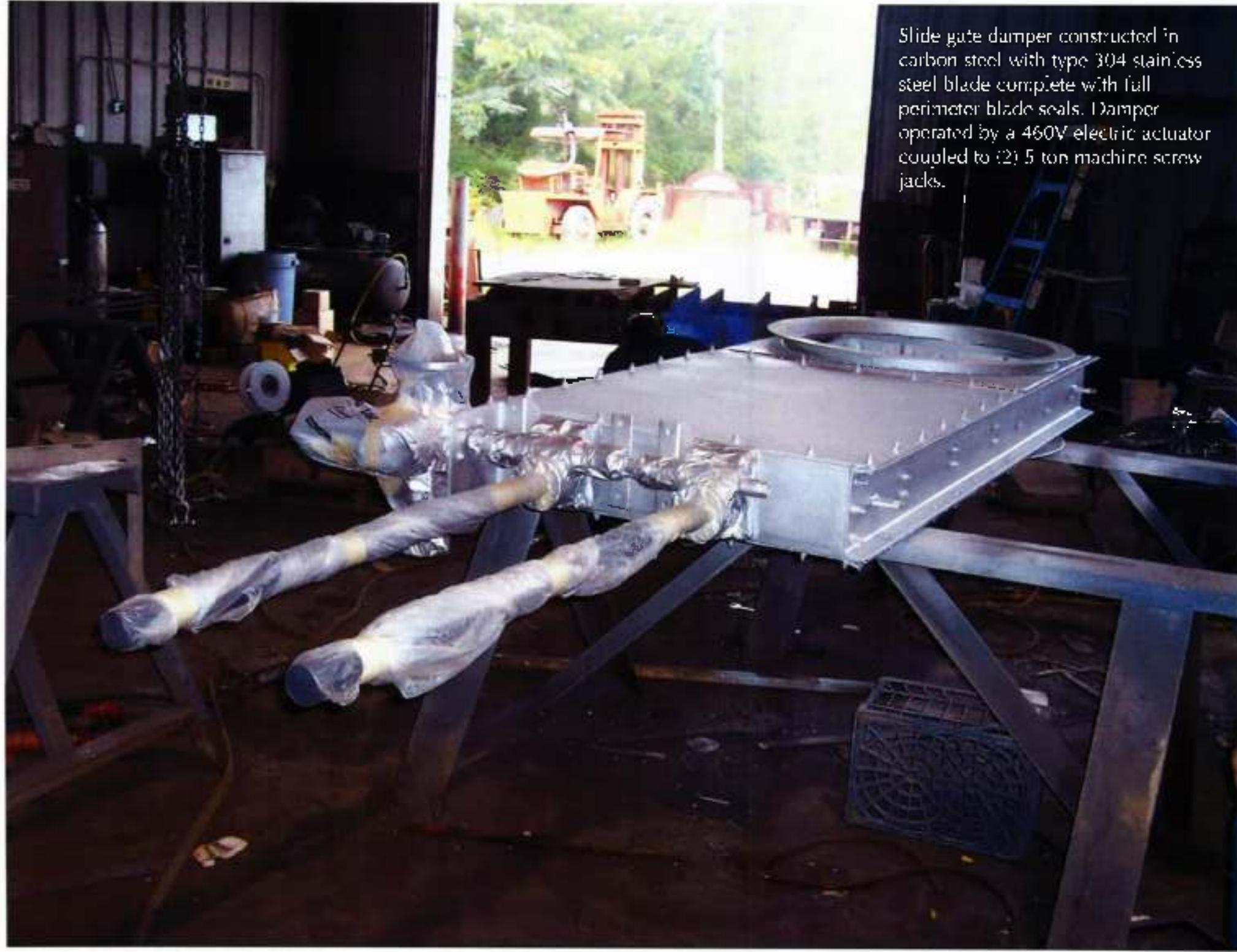
Slide gate damper constructed in carbon steel with type 304 stainless steel blade complete with full perimeter blade seals. Damper operated by a 460V electric actuator coupled to (2) 5 ton machine screw jacks.
