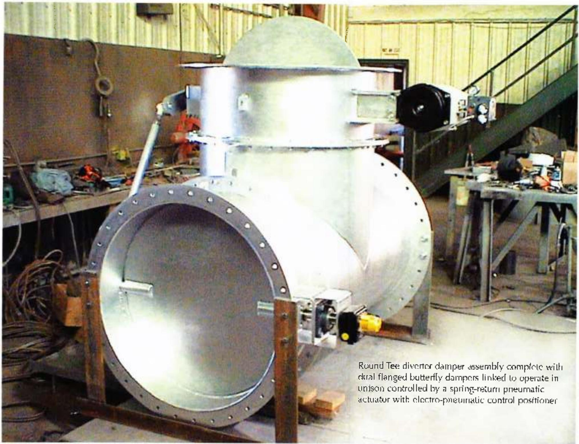
Round Tee diverter damper assembly complete with dual flanged butterfly dampers linked to operate in unison controlled by a spring-return pneumatic actuator with electro-pneumatic control positioner
