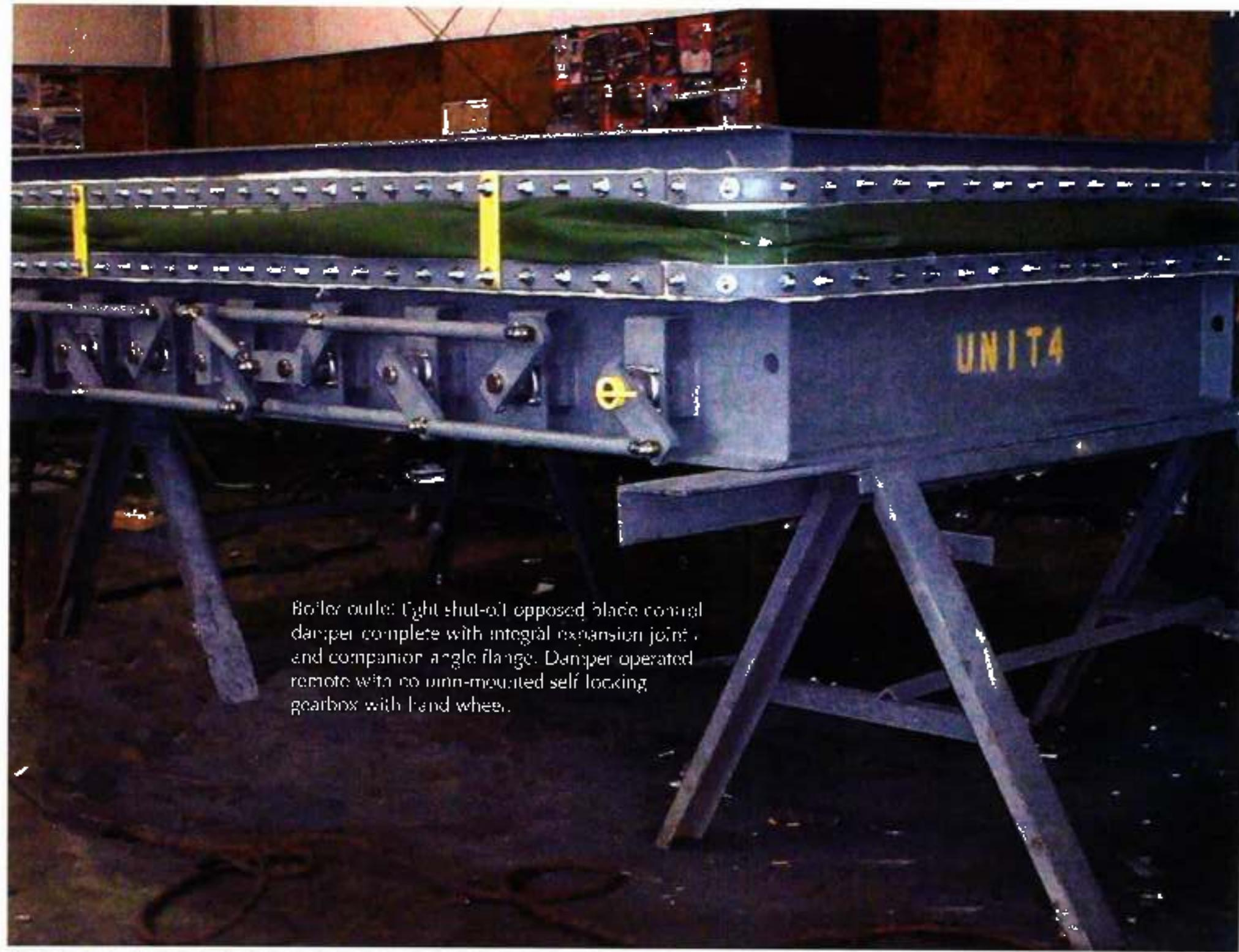
Boiler outlet tight shut-off opposed blade control
