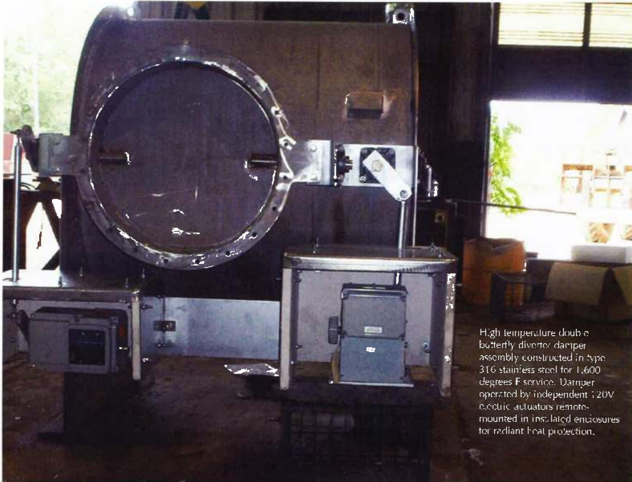
High temperature double butterfly diverter damper assembly constructed in type 316 stainless steel for 1,600 degrees F service. Damper operated by independent 120V electric actuators remote-mounted in insulated enclosures for radiant heat protection.
