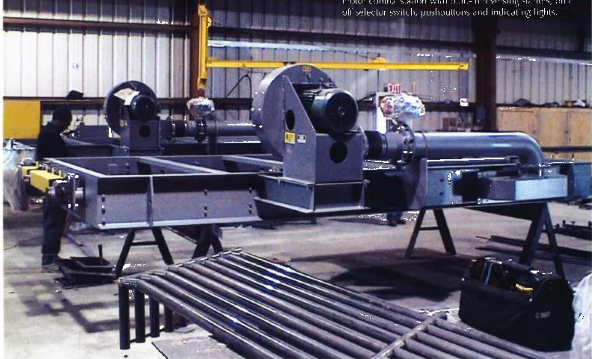
Coal handling slide gate isolation slide gate damper designed to isolate inlet holding silo from outlet rotary valve. Damper designed to pull through coal build-ups in order to perform maintenance on lower outlet equipment. Damper complete with electric actuator with local motor control station with built-in reversing starters, on / off selector switch, pushbuttons and indicating lights.
