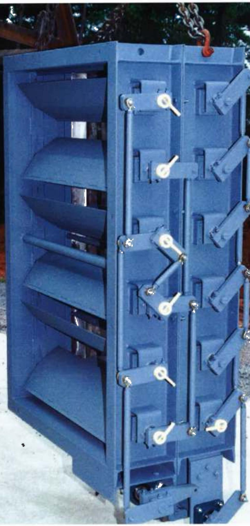
Face outlet tandem lower dampers consisting of enclosed blade control damper for motivation connected to existing Beck actuator and tight shut-off parallel blade isolation damper with full perimeter blade seals and bottom purge air chamber for seal air connection.
